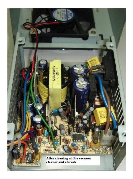
As you know, we as electronic repairers can't just see things at only one side; we have to see the surrounding areas too. What I meant was, try to see if there are any suspicious components that contributed to the failure of the power supply such as broken components, dry joints, loose connection, decayed glue and etc before start checking the suspected area.
