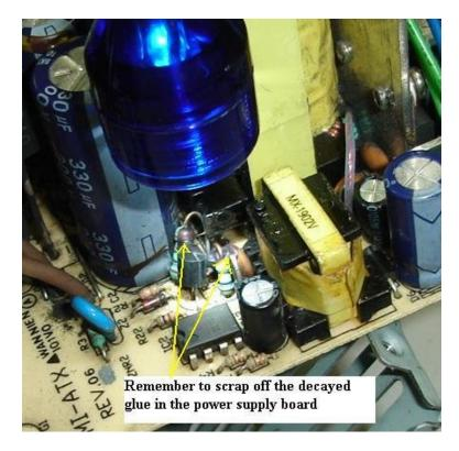
What I saw was at the primary side there were some components covered with decayed glue as seen in the picture. I have to carefully remove it by scrapping off the layers of the decayed glue while preserving the outer layers of the components. Once it was done, I cleaned it with the Thinner solution. Decayed glue could cause serious or intermittent problem in electronic equipment because it can be conductive.
