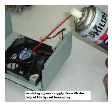
If you repair any ATX power supply, make sure you check the fan too because some power supply failure was due to heat caused by a faulty fan. The purpose of the fan is to suck out all the heat generated by the components inside the power supply especially the switch mode transformer and Schottky diodes that were attached to a heatsink. In order for the fan to run smooth, you can service it by using a Philips oil base spray as shown in the photo.
