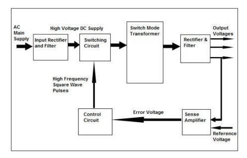
If you look at the block diagram from the previous page, if there is no load connected to the power supply, the sense amplifier will send an error voltage to the control circuit and this control circuit will turn off the switching circuit. If the switching circuit is not functioning thus there will be no output voltage because the switch mode transformer is not working.
