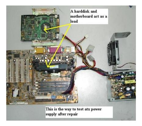
The reason I tested it on a junk motherboard first so that it would not cause the good motherboard (in the CPU) to go bad just in case if the power supply output voltages were still high. Better safe than regret later. **By the way you can't test an ATX power supply without load otherwise it may turned On for a while and then shut down.** This is because, without load the output voltages produced will become very high and this will trigger the protection circuit to shut down the power supply.
