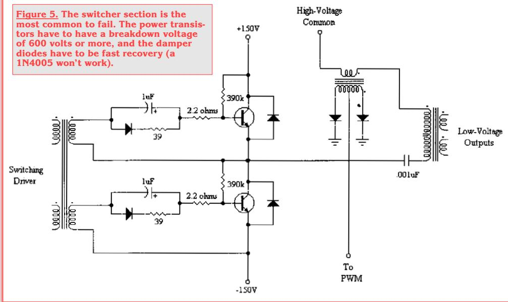
**Figure 5.** The switcher section is the most common to fail. The power transistors have to have a breakdown voltage of 600 volts or more, and the damper diodes have to be fast recovery (a 1N4005 won't work).
