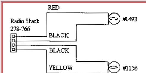
Figure 2. A dummy load can be made from a couple lamps that you can buy at any auto parts store and an extension cable from Radio Shack.
