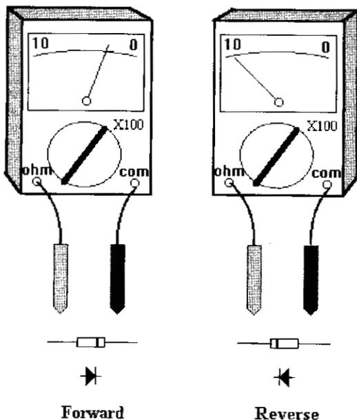
**Figure 7. A cheap VOM is the best way to check transistors and diodes. Why? Because the test voltage has to be enough to breach the barrier voltage of a silicon diode, typically 0.7 volts, and a lot of DVMs have a probe voltage of 0.3 volts and less.**
